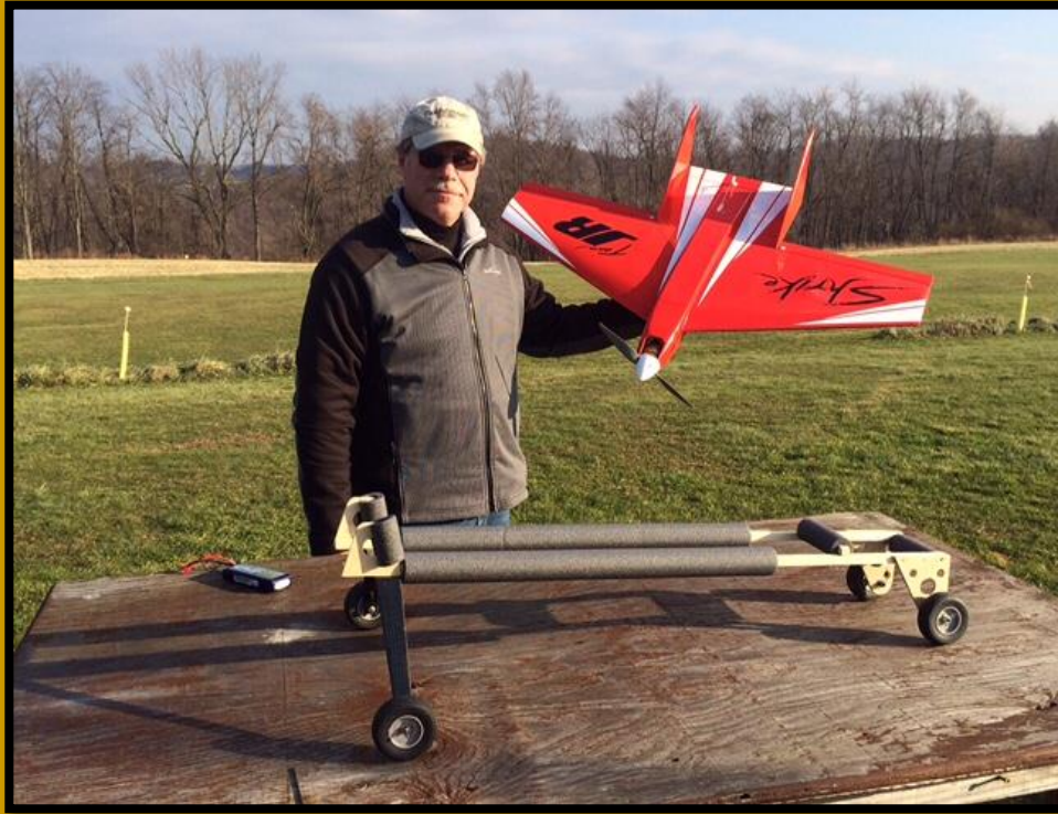
View of wheeled dolly used during take off of the Shrike. Ron's custom design.
