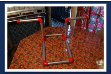
Center of Gravity Stands constructed, painted, and cemented to your specifications. Standard stands are 18 ½ inches long, 11 ½ inches wide, and 12 inches high. The center of gravity posts are 11 inches apart and can be swung out to 22 inches apart. The stands are constructed using ¾ inch pvc pipe, painted to your specifications, and then cemented. The paint I use is Rustoleum High Intensity plastic paint. The stands are priced at \$25.00 per stand.
