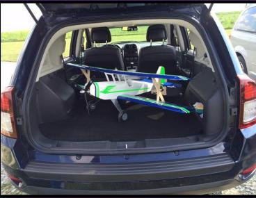
Well, Bill has been busy again scratch building this biplane named "Flybaby". He started with downloaded Russian plans from the Internet. He reduced the much larger plan design down to a 53" wingspan that is the magic number for the fully assembled aircraft to fit in his SUV. He is using an Eflite 60 brushless motor with a 14x10 three blade prop. Power is from a six cell 5000mah Lipo pack. Bob Haden assisted with the successful maiden flight.
